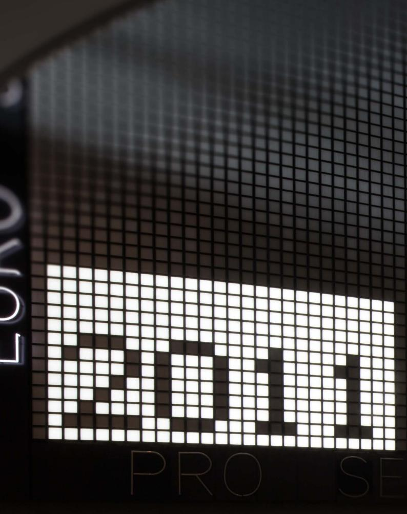
Eye catcher and information center in one: 5,670 monochrome LED Tiles from Schnick-Schnack-Systems illuminate a surface of 80 square meters and are able to transport company content. The diffusors imitate the product that is responsible for MANN + HUMMEL'S rise to a global player: the filter. The completion of this ambitious project took nearly two years.
